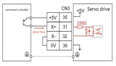
• The wiring of Y+ (33 feet) and Y- (34 feet) is the same as that of X+ and X-.
