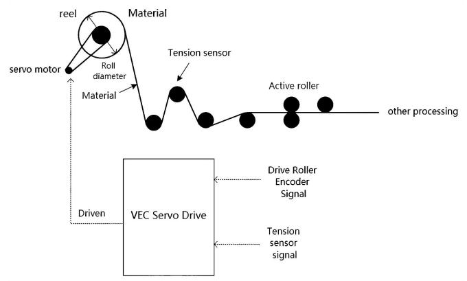
VEC servo integrates 4 tension control modes, namely closed-loop speed mode, closed-loop torque mode, closed-loop speed/torque automatic switching mode, and
