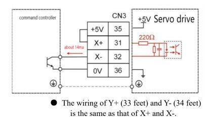
b. When using an external power supply prepared by the user:
