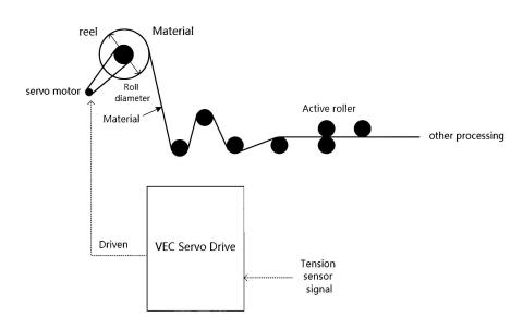
Before use, it is necessary to set the basic application parameters, including the number of pulses per meter of feed, the number of pulses per revolution of the reel, the given source of tension and other related parameters, and the related parameters of rolling diameter calculation.
