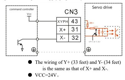
② The upper controller is PNP type (European PLC such as Siemens)a. When using the drive's internal 5V power supply:
